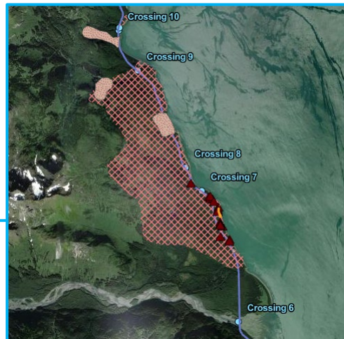
Sinkhole and rockfall hazards between crossings 6 and 10
